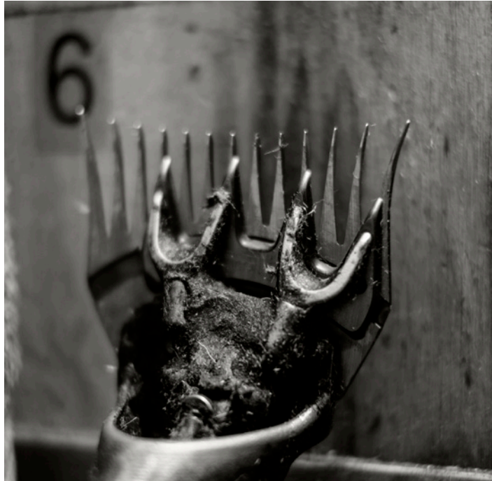
The shearer's indispensable tools: Shearing moccasins and electric shears. The shears are regularly cleaned and taken well care of in order to function optimally for sheep and wool. The moccasins are soft and gentle for both the shearer and the sheep.
